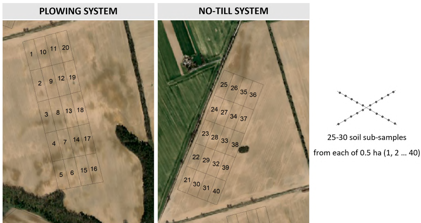
Fig. 2. Scheme of sample points corresponding to the fertilization gradient and controls in two fields dedicated to plowing and no-till maize cultivation together with the patterns of collection of sub-samples from each 0.5-ha area.
