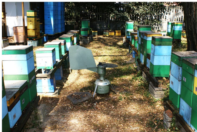
Figure 3. Experimental procedures. A Hirst-type spore trap was placed among the hives.
